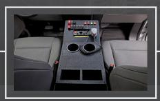
POLYUREA SPRAYED ALL ALUMINUM FRONT CONSOLE - INTERCHANGEABLE DESIGNS
